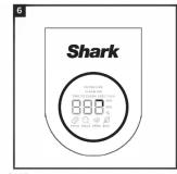
6. When the unit is powered on, it will begin to analyze the air quality indicated by the rotating lights. After a few seconds the unit will display the current air quality.
