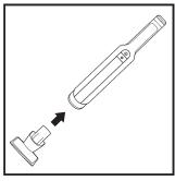
To attach an accessory to the hand vacuum, slide it into the opening in the nozzle. To remove the accessory, slide it off the nozzle.
