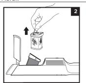
2. Hold the filter housing over a trash receptacle. Lift the fabric filter by the metal ring to remove it from the housing. Tap lightly to remove any dust and debris, then rinse with water only. Let the filter air-dry for at least 24 hours or until completely dry before reinstalling.
