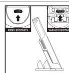
Plug the charging dock into a wall outlet. Charge the vacuum by sliding it into the charging dock nozzleMake sure the contacts on the vacuum are aligned with the contacts on the charging dock.
