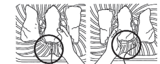
Correct thermometer placement. Thermometer grip is fully inside unit.
