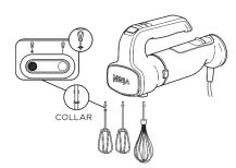
Attach both beaters, the whisk using the accessory slots on the mixer head. Insert the beater with the collar into the slot with the diagram showing a collar. The whisk can be inserted into either slot. You will hear a slight click when locked in place.
