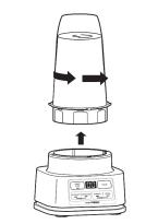
Remove the cup from the motor base by turning it counterclockwise and then lifting up.
