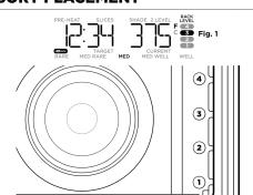
The oven has 4 available rack positions where your accessories can slide into the unit (see image above). When you select a function, the corresponding rack number(s) will illuminate on the control panel. The numbers on the control panel (see Fig. 1) will coincide with those on the interior of the unit.
