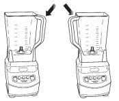
4 The pitcher can be placed on the motor base two ways; the handle can be on the front right corner or the front left corner.
