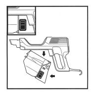
To remove the dust cup from the handheld vacuum, press the two **Dust Cup Release** buttons at the same time and slide out the dust cup
