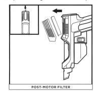
To access the post-motor filter, press the release latch on the filter cover on the handheld vacuum. Remove the cover and lift out the filter.
