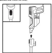
Press the Wand Release button and lift off the handheld vacuum
