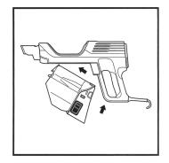
To reinstall, push the lid closed, then insert the front end of the dust cup into the handheld vacuum first, then the back end, until it clicks into place.
