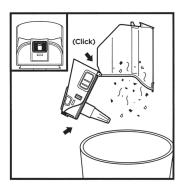
Hold the dust cup over the trash. Press the **Empty** button and pull open the dust cup lid until it clicks and locks in the open position. Gently tap the cone-shaped screen inside the dust cup to knock dust and debris into the trash
