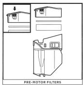
With the dust cup detached, press the Filter Access buttons on both sides of the back of the dust cup, then pull out the filter housing. Pull the foam filter out of the housing, then lift out the felt filter by the pull tab
