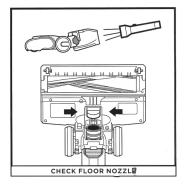
Detach the wand, then tilt the floor nozzle Debris Intake back and check openings for blockages.
