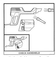
Remove the handheld vacuum from the wand and check all dust cup intake openings for debris or blockages
