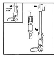
Press the Wand Release button near the top of the wand to detach the handheld vacuum Align the Catch on the side of the handheld vacuum with the Storage Hook on the wand, then hang the handheld vacuum from the hook
