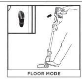
To clean floors, step on floor nozzle and tilt handheld vacuum back
