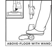
For more reach, detach the wand, Stand the vacuum upright, step on the Foot Pedal on the side of the nozzle, and pull up the wand to detach.
