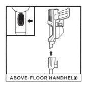
To detach the handheld vacuum, press the Wand Release button and lift the handheld vacuum off the wand. Great for cleaning stairs, furniture, and
