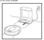
When the cleaning cycle is complete, or if the battery is running low, the robot will search for the base. If your robot doesn't return to the base, its charge may have run out.
