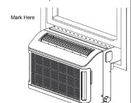
Remove adhesive backing from the Side Pane Brackets. Place them onto unit so that the front edges are lined up with the drawn line as seen
