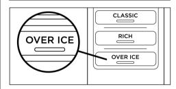
To start a brew, press OVER ICE. The brew will begin, stop, and pause for a short period of time before it begins again. This process ensures even saturation of the coffee grounds. The unit will beep when the brew has completed.
