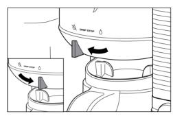
When brewing a carafe, close the **Drip Stop** to pause the brew cycle and pour a cup. Promptly replace the carafe and open the Drip Stop to complete the brew.
