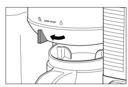
When the brew cycle is complete, set the Drip Stop to the closed position to stop dripping from the brew basket. While the Drip Stop is closed, the Drip Stop indicator will illuminate.
