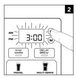
Quickly press the hour (H) and/or minute (M) buttons to increase the time up to 4 hours or decrease the time to 0 hours. Press **STAY WARM** to set the new time. The brewer will automatically save the new time after 5 seconds of inactivity.
