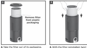
3. With the filter reinstalled, twist the filter door until it clicks into place.
