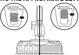
The Rocket<sup>™</sup> has a 2-speed Power slider switch on the handle to select the speed of the brushroll.. Slide the switch to appropriate speed setting (I or II) and start cleaning
