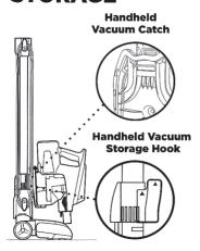
Press the Wand Release button on the top of the wand to release the handheld vacuum. There is a catch on the bottom of the handheld vacuum. Hang it from the hook located on the bottom portion of the wand. Wrap the cord around the two cord hooks.
