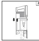
To empty the Dust Cup while it is attached to the handheld vacuum, position the dust cup over a trash receptacle and slide the CleanTouch™ Dirt Ejector slider forward.
