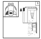
To remove the dust cup from the handheld vacuum, press the **CleanTouch Dust Cup Release** button near the handheld vacuum nozzle. Tilt the dust cup and lift off to remove.
