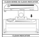
The Clean Indicator visually confirms when floors are clean. When the unit senses heavy debris, suction will increase for more cleaning power. When the debris is cleared suction will decrease. The clean indicator displays the level of debris detected. For best use, wait until the indicator returns to its lowest level before moving to the next area
