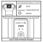
Press the ( ) button to toggle between ECO, Clean Sense IQ, and Boost modes. To save battery power, select ECO mode. For everyday cleaning power, select Clean Sense IQ mode. For an extra burst of power, select
