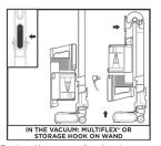
the vacuum for charging, press the MultiFLEX Wand Unlock Latch while folding the handheld vacuum forward until the wand clicks and locks, or hang the handheld vacuus from the storage hook on the wand. Plug the charger into the charging port on the handheld
