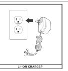
Plug the Li-Ion Charger into a wall outlet
