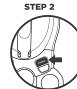
2 Press POWER to clean hard floor surfaces, area rugs or above-floor. The brushroll will not spin in this mode.
