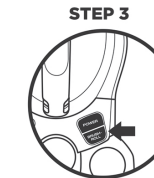
3 Press POWER and BRUSHROLL to clean carpets. The BRUSHROLL button will illuminate green. The brushroll will spin only when the vacuum is reclined and the BRUSHROLL button is green.
