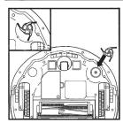
Snap the included Side Brush onto the square peg on the bottom of the robot.
