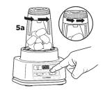
NOTE: While processing, twist the Power Paddle counterclockwise continuously.
