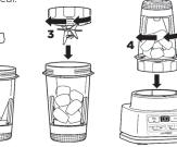
4 Turn the bowl upside down and install on motor base by aligning the tabs on the bowl with the slots on the base. Then, rotate bowl clockwise until it clicks. Once locked in place, the programs will illuminate and the unit will be ready for use.
