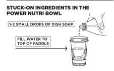
For stuck-on ingredients, such as nut butter, rinse the bowl and blade assembly under warm water.
