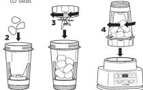
4 Turn the bowl upside down and install on motor base by aligning the tabs on the bowl with the slots on the base. Then, rotate bowl clockwise until it clicks. Once locked in place, the programs will illuminate and the unit will be ready for use.
