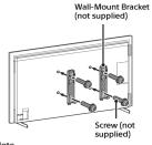
If using an electric screwdriver, set the torque at approximately 1.5 N·m {15 kgf·cm}. XR-75X901 / 75X90C1 / 65X901 / 65X90C1 /
