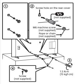
The length of the M6 machine screw differs depending
