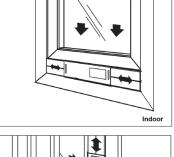
Place the Air Conditioner close to the window ensuring there is at least 20" of clearance from the wall and any other obstructions. Extend the hose so that it reaches the Window Kit. Insert the Exhaust Hose Adapter into the opening in the Window Kit and slide it into the locking position. Ensure that the hose runs straight to the window with no excess extension. Use the small screw to attach the exhaust hose assembly to the window sealing plate assembly.
