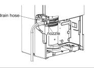
3. Thread a garden hose (not supplied) onto the nozzle, cut to length, and lead it to the floor drain
