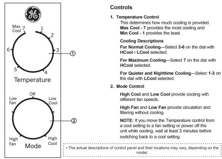
This determines how much cooling is provided. Max Cool - 7 provides the most cooling and Min Cool - 1 provides the least.
