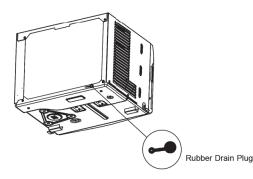
Removing this plug will lower the Energy Efficiency of your until. NOTE: Do not drill hole in the base pan.
