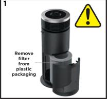
You must set up the filter before operating. First, remove the filter cover and filter from the back of the air purifier. Then, take the filter out of its sealed plastic packaging.
