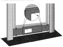
7. Using one pointed screw, install the Security bracket to the window.
