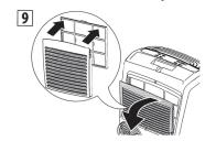
Use a vacuum cleaner to remove the dust collected on the filter. If it is very dirty, immerse in warm water and rinse a number of times. The water should never be hotter than 104°F (40°C). After washing the filter, allow it to dry completely before repositioning it.
