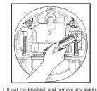
Reinstall the brushroll, inserting the flat end first. Close the brushroll access door and press down until both sides click into place.
