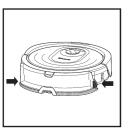
When mopping is complete, remove the reservoir by pressing both buttons and sliding it out. Empty the reservoir after each use.
