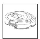
When the reservoir has fluid and is properly installed, with the mop pad attached, the robot is ready to vacuum and mop simultaneously. Press the Clean button on the robot or in the app to start a vacuumin and mopping run. The robot will prime the mop pad for 30 seconds before starting its run.
