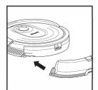
Firmly push the reservoir into the back of the robot hehind the dust hin, and ensure both latches click into place. The water droplet icon on the robot will illuminate white when the reservoir is insert properly.
