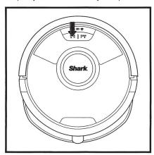
To turn ON the robot, press and hold the DOCK button for 5-7 seconds. To charge, place the robot on the dock. The robot will beep when charging begins and the charging indicator on the dock will turn from green to blue.
