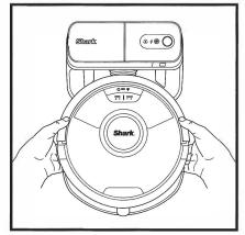
If the robot has no charge or it cannot return to the dock, manually place it on the dock. The indicator light will turn blue and the robot will beep when it is correctly placed on the dock. If the Vac & Mop Dust Bin is inserted, your robot will dock forward to prevent the wet pad from touching the charging contacts.
