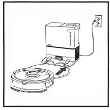
When the cleaning cycle is complete, or if the battery is running low, the robot will search for the dock. If the robot doesn't return to dock, its charge may have run out, or if it is in wet cleaning mode, the dock may be blocked by carpet.
