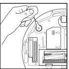
Carefully unwind and remove any string or hair wrapped around brushes. Gently wipe brushes with a dry cloth. To reinstall, snap the brushes over the pegs. Spin the brushes manually to make sure they are installed correctly.
