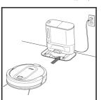
When the cleaning cycle is complete, or if the battery is running low, the robot will search for the base. If you is running low, the robot will search for the base. If you robot doesn't return to the base, its charge may have run out. Make sure that all the protective film has been removed from the base, and recharge the robot
