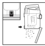
Press lower release button to open bottom of dust cup.
