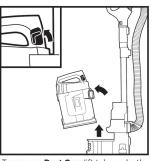
To remove **Dust Cup**, lift tabs on both sides of dust cup handle. Tilt dust cup forward, then lift to remove
