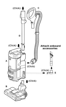
NOTE: For proper operation, ensure all parts are firmly CLICKED into place.
