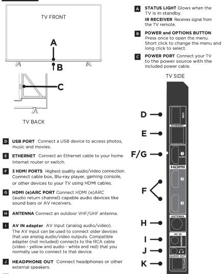
к **OPTICAL (DIGITAL AUDIO OUT)** Connect an optical cable to an external digital audio system.
