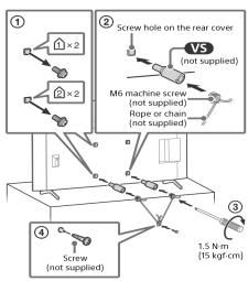
The length of the M6 machine screw differs depending on the rope or chain diameter. Please refer to below
