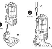
Insert canister into motorized floor nozzle.
