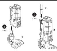
Insert canister into motorized floor nozzle
