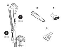
Connect handle to the wand, pressing until it clicks into place. Connect hose to the back of the canister pressing until it clicks into place.
