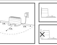
Place the charging dock on a level surface with its back against a wall, in a space without obstructions, that can easily be accessed by your robot. Remove any objects that are closer than 3 feet (1 meter) from either side of the dock, or closer than 5 feet (1.52 meters) from the front of the dock. Plug the **Charging Adapter** it starts charging on the dock
