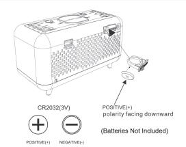
The lithium backup battery needs replacement when the LOW BATTERY indicator flashes, otherwise, the time and alarm settings will be lost/reset
