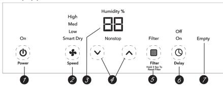
Controls NOTE: When the bucket is full or removed, the controls cannot be set.
