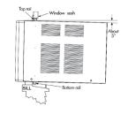
C. Install the side bracket into the unit and into the window sill using two 1" wood screws provided.
