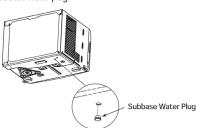
To ensure maximum efficiency it is recommended to check to ensure the rubber drain plug is properly inserted. This plug may be removed during operation to minimize water in the back of the unit; however, removing it will lower the efficiency of your unit.
