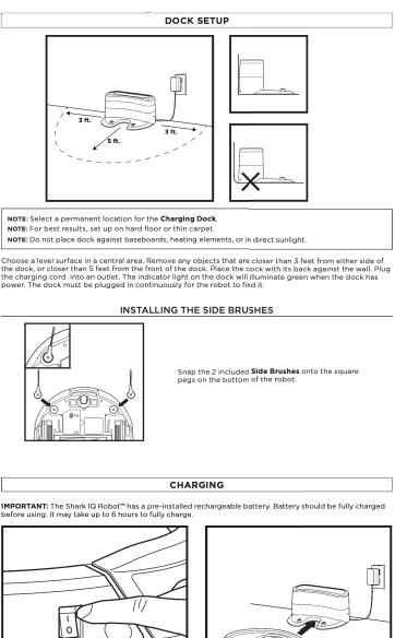
When the cleaning cycle is complete, or if the battery To charge, the **Power** button on the side of the robot nust be in the ON position (1). The robot will been is running low, the robot will search for the dock. when charging begins. If your robot doesn't return to the dock, its charge may have run out.
