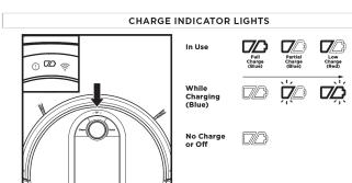
The blue indicator lights on the robot show how much charge is remaining While the robot is charging, both blue LED lights will flash. When charging is complete, both blue lights will illuminate steadily. It may take up to 6 hours to fully charge your robot.
