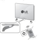
Power Off<sup>1)</sup> (Press and Hold) Menu Control (Press<sup>2)</sup>) Menu Selection (Press and Hold<sup>3)</sup>
