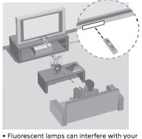
remote control; try turning off the fluorescent lamps.
