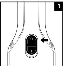
Make sure to switch the unit into the "O" position to power off before charging.
