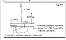
Check your storm windows - if your storm window frame does not allow the clearance required, correct by adding a piece of wood as shown in Fig. 17, or by removing storm window while room air conditioner is being installed.
