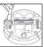
Periodically clean the drive wheels and the housing around them. To clean, rotate each wheel while dusting.
