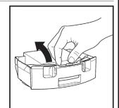
To avoid spills, be sure to hold the dust bin in an upright position. Pinch and lift to open the lid.
