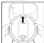
If the robot has no charge and cannot return to the base, manually place it on the base. When the robot evacuates dust and debris into the base, the blue light on the base will be solid blue. Once charging starts, the robot will beep and the blue light on the base will pulse.
