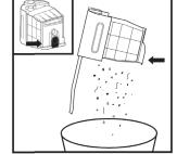
To empty the bin, hold it over the trash, then press the release button with the trash can icon on the bottom of the bin. The bin I did will open, releasing dust and debris. Lightly tap the dust bin against the insite of the trash receptacle to knock off any remaining debris. Reinstall the bin by sliding it into the slot in the base until it clicks into place.
