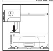
There are 2 indicator lights on the front of the base, the green power indicator light and the blue charging indicator light. When the base is plugged in and the power switch is turned on, the GREEN power light © will illuminar. By then the robot is charging on the base, the BLUE light will pulse. When charging is complete, the
