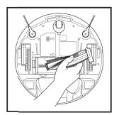
Lift out the brushroll, and clean off any debris. Reinslall the brushroll, inserting the flat end first Close the brushroll access door and press down both sides click into place.
