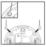
nap the 2 included **Side Brushes** located in the ad packaging, onto the square pegs on the botto f the robot.
