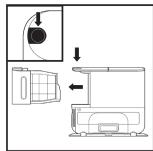
The **Base Dust Bin** holds up to 30 days' worth of dust and debris. Empty the bin when the debris level approaches the max fill line. To detach the bin, press and hold the **Release** button on the top and slide out the bin.
