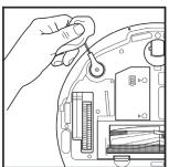
Carefully unwind and remove any string or hair wrappad around brushes. Gently wipe brushes with a dry cloth. To reinstall, snap the brushes over the pegs. Spin the brushes manually to make sure they are installed correctly
