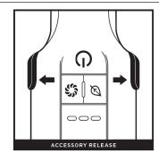
If your vacuum has One-Touch Accessory Release buttons, press the **One-Touch Accessory Release** buttons on either side of the handle to release an accessory from the hand vacuum.
