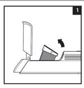
With the dust cup removed and the power off, pinch both sides of the filter housing and pivot it upward to access the filter.
