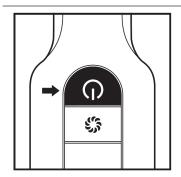
Press the **On/Off** button on the handle to go into Deep Clean mode. Press the power button again to turn off the vacuum.
