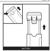
To remove the battery from the hand vacuun press the release tabs on the battery cap and slide out the battery. To reinstall, slide the battery into the compartment in the handle until it clicks into place
