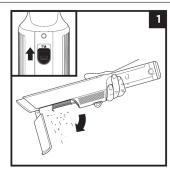
With the power off and the hand vacuum positioned over a trash receptacle, slide the Dust Cup release button near the handle, and the dust cup will drop open. Tap the filter screen lightly to knock off dust and debris.
