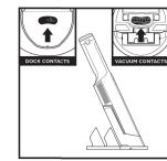
Make sure the contacts on the vacuum are aligned with the contacts on the charging dock.
