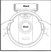
If the robot has no charge or it cannot return to the dock, manually place it on the dock. The indicator light will turn blue and the robot will beep when it is correctly placed on the dock
