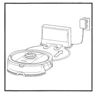
When the cleaning cycle is complete, or if the battery is running low, the robot will search for the dock. If the robot doesn't return to dock, its charge may have run out, or if if it is in wet cleaning mode, the dock may be blocked by carpet.
