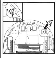
Snap the included **Side Brush** onto the square peg on the bottom of the robot.
