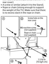
The length of the M6 machine screw differs depending on the rope or chain diameter
