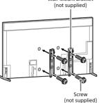
If using an electric screwdriver, set the torque at approximately 1.5 N·m {15 kgf·cm} Detaching the Table-Top Stand from the TV remove the screws 4.
