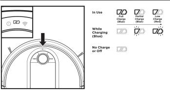
The blue indicator lights on the robot show how much charge is remaining While the robot is charging, both blue LED lights will flash. When charging is complete, both blue lights will illuminate steadily. It may take up to 6 hours to fully charge your robot
