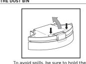
dust bin in an upright position. Use the finger slots to open the lid.
