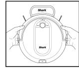
If the robot has no charge and cannot return to the dock, manually place it on the dock. The dock indicator light will flash blue and the robot will beep when charging begins.
