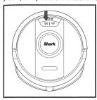
To turn ON the robot, press and hold the DOCK button for 5-7 seconds. To charge, place the robot on the dock. The robot will beep when charging begins and the charging indicator on the dock will turn from areen to blue.
