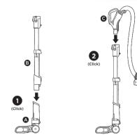
Insert wand into motorized floor nozzle.
